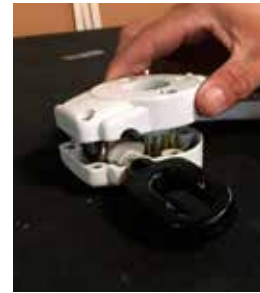
⑤ Remove the Gear Box cover. Keep all parts intact.
