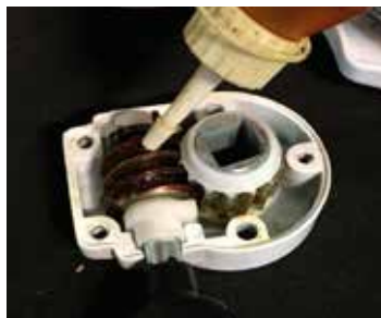
⑥ Lubricate the Gear Box threads. Place the Gear Box cover back on and secure with 3 screws.
