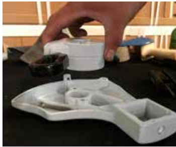
③ Remove the Gear Box from the Cassette cover. Lay the Gear Box on a flat surface.
